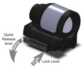
2.Once the mount is fully seated on the rail, lock the optic by closing the lever. An audible click is heard when the mount is locked and when the quick release lever is closed. Attempt to release the quick release lever without pushing the lock lever to ensure positive lock.
